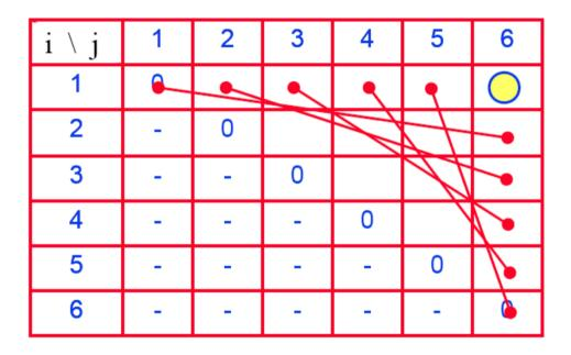
$$\begin{split} m[1,6] &= \min_{1 \leq k < 6} \{m[1,k] + m[k+1,6] + c_0 \cdot c_k \cdot c_6\} = \\ &= \min \{m[1,1] + m[2,6] + c_0 \cdot c_1 \cdot c_6 \ , \ m[1,2] + m[3,6] + c_0 \cdot c_2 \cdot c_6 \ , \\ &\qquad \qquad m[1,3] + m[4,6] + c_0 \cdot c_3 \cdot c_6 \ , \ m[1,4] + m[5,6] + c_0 \cdot c_4 \cdot c_6 \ , \\ &\qquad \qquad m[1,5] + m[6,6] + c_0 \cdot c_5 \cdot c_6\} \end{split}$$
