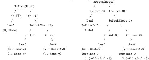
(Root.0) is called an *accessor*, that represents the access path to a value that can be reached by deconstructing the scrutinee. In this example Root.0 is the first subvalue of the scrutinee.
