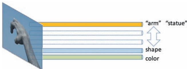
Figure 1.3. Any media object can be seen as a collection of channels of information; some of these information channels (such as color and shape) are low-level (can be derived from the media object), whereas others (such as semantic labels attached to the objects by the viewer) are higher level (cannot be derived from the media object without external knowledge).
